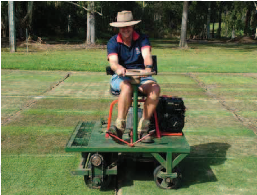
Plate 4.1. Self-propelled modified Brinkman Traffic Simulator for applying simulated turfgrass wear.
